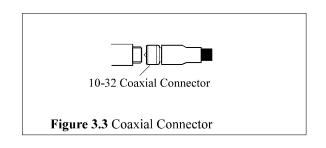
Plug the male connector on the cable into the mating female connector on the sensor. Then, holding the sensor stationary, secure the connector in place by tightening down the attached cable sleeve. See Figure 3.3.
